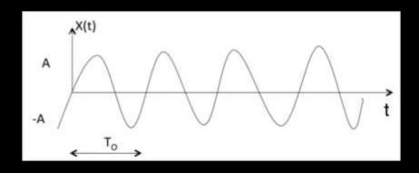
The signal shown in the above image will repeat for every time interval  $T_o$  (therefore it is periodic with the time period  $T_o$ .)
